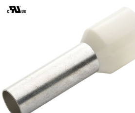
Figure 4 : Embout terminal 0,5mm 2 , Blanc, 14mm, Lot de 100 pièces, RND Connect
