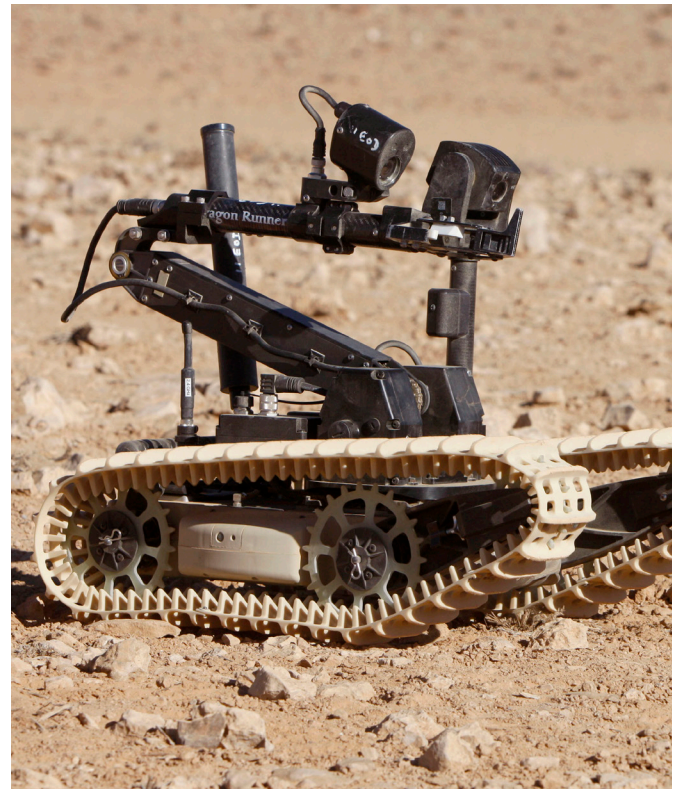
The lightweight Dragon Runner Bomb Disposal Robot is easy to transport and can be deployed in many different terrains (courtesy of Crown)
