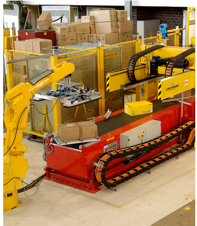
One of DHL's robots is capable of optimally loading a shipping box with packages (courtesy of DHL Express)
